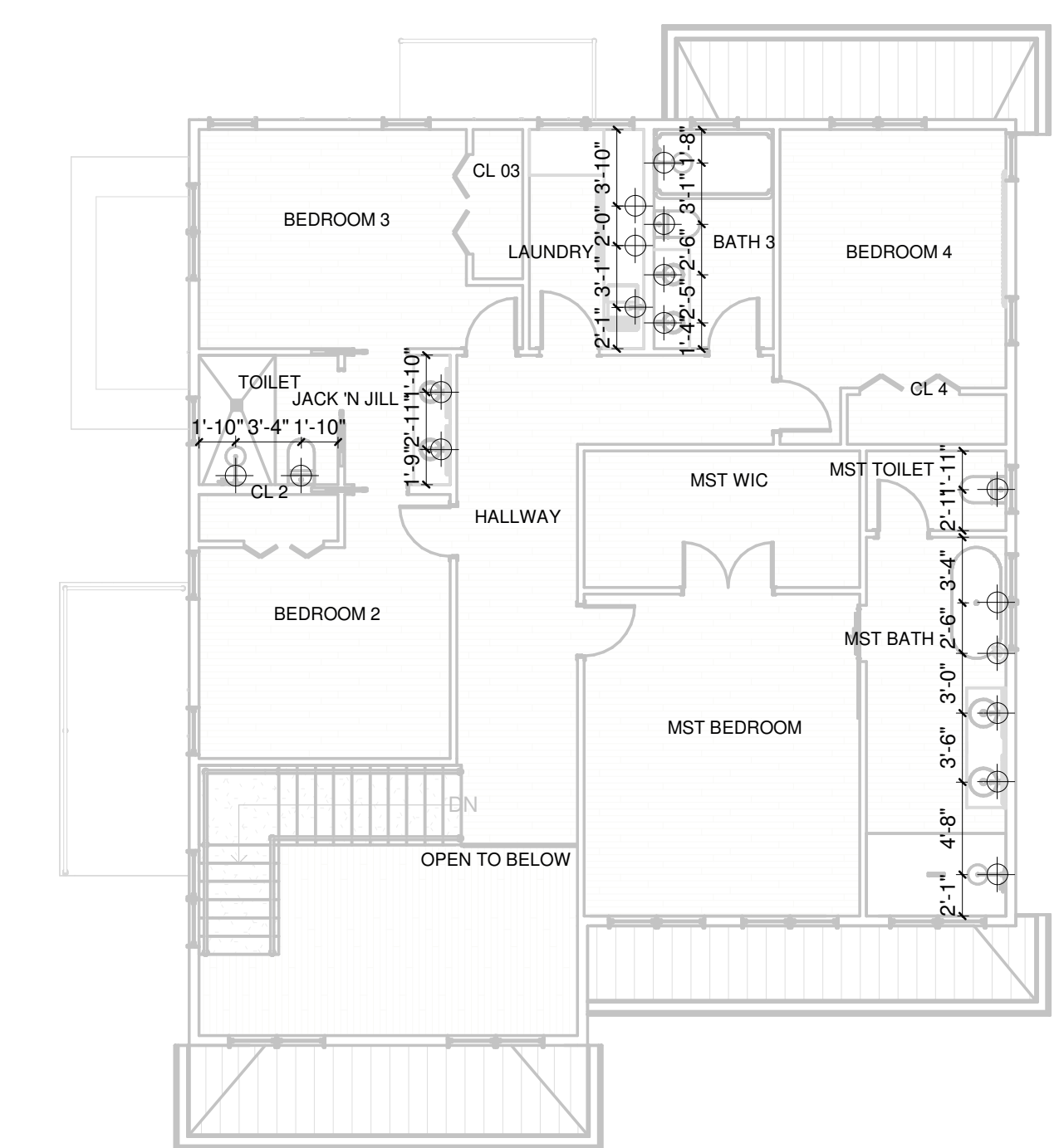
3 PLUMBING SECOND FLOOR PLAN SCALE: 1/8" = 1'-0"
